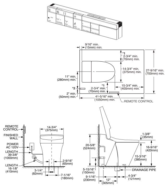
NOTES: This bidet toilet is designed to rough-in at a minimum dimension of 12" (305 mm) from finished wall to C/L of outlet.
